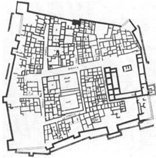
Plan of Marisa (Tell Sandahanna), a typical Hellenistic city, almost square, with streets intersecting at right angles and buildings surrounding an open court in each block (F. J. Bliss and R. A. S. Macalister)
